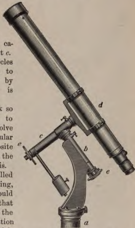
FIG. 41.—A simple equatorial mounting.
